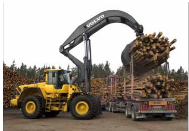
For stacking or loading, Volvo’s L180F High Lift offers an 8.6 tonne working load and 5.8 metre lift height under the closed grapple.
